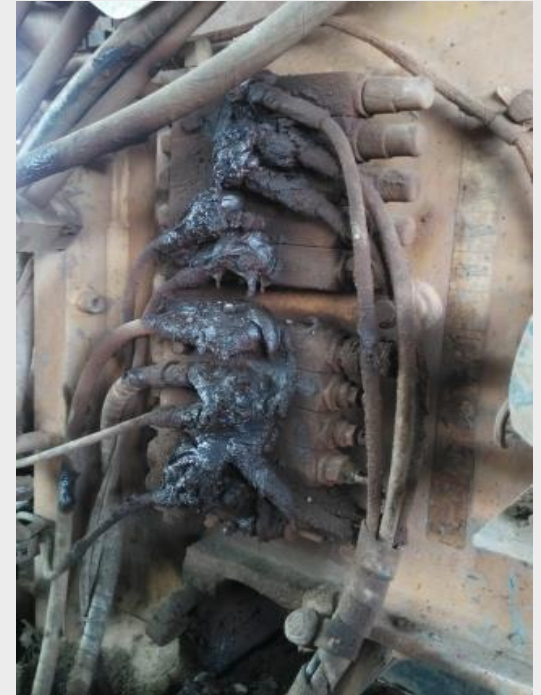
Leaking grease injectors
