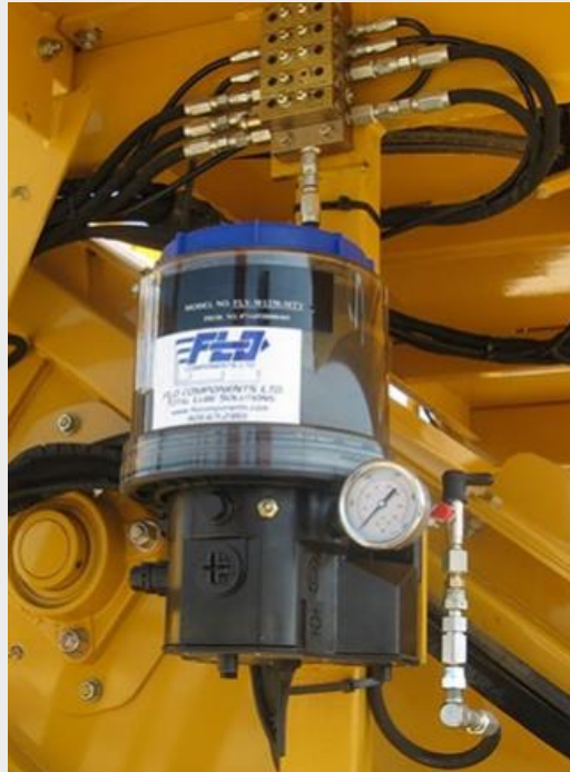
Automatic grease lubrication system
